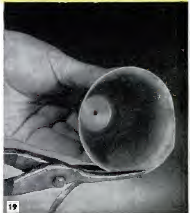
Metal spun over high form tends to stretch. Edge usually must be trimmed before spinning to final shape
